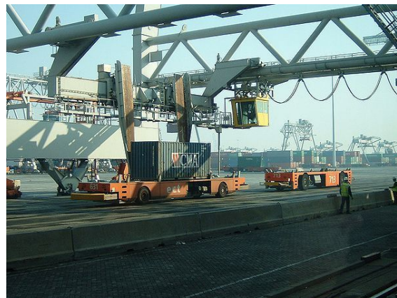
Unmanned vehicles handle containers at Europe Container Terminals (ECT), the largest container terminal operator in Europe.
